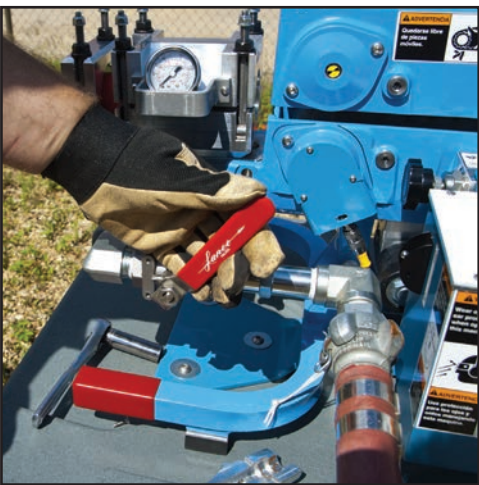
Figure 69. Turn On Air
