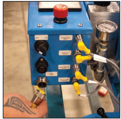
Figure 62. Attach Power Cord
