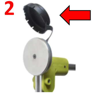
2 Uncover Magnet and Position Onto Transformer Lid.
